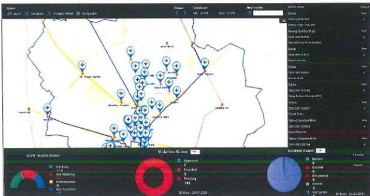
Figure 4:20 – Indicative Screen of Video Wall GUI (Notification Windows)
