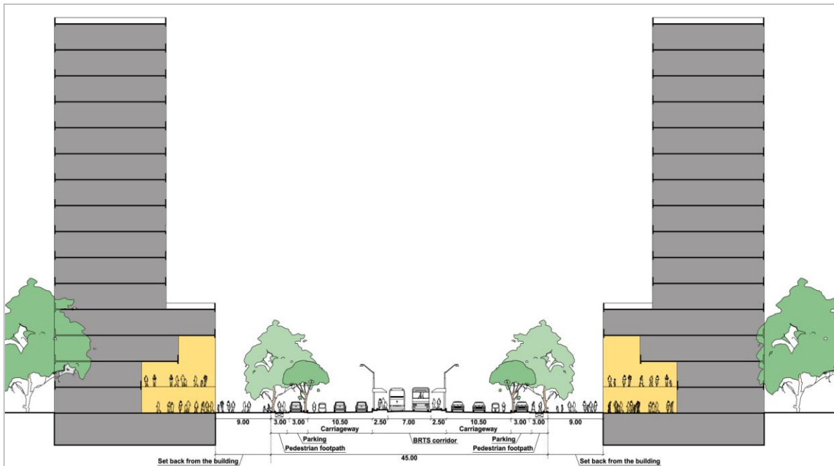
Figure 35: Proposed 45m. wide Road Section – Central Mass Transport Bay - Surface
