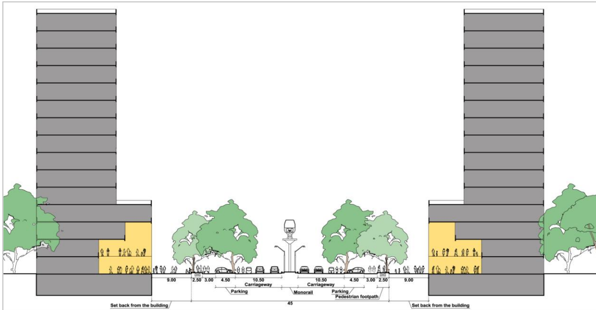
Figure 35: Proposed 45m. wide Road Section – Central Mass Transport Bay - Surface
